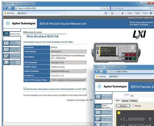
Agilent B2900A is accessed easily by IP address.
