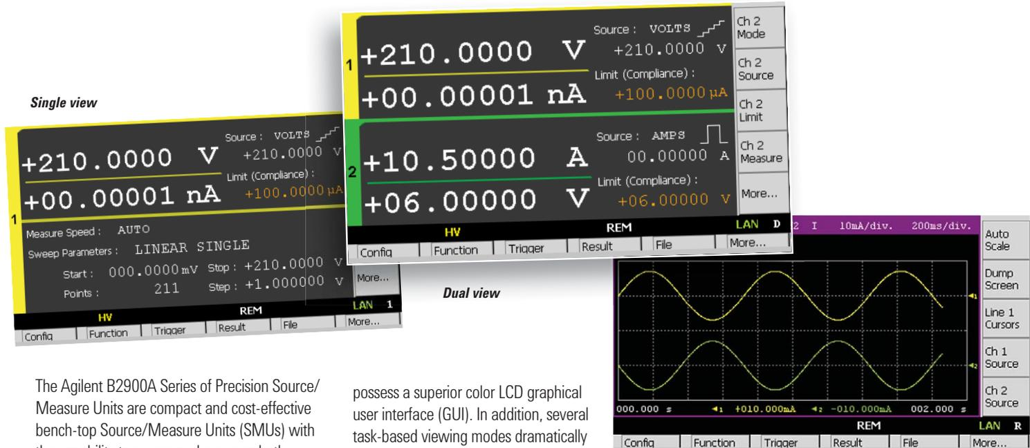
The Agilent B2900A Series of Precision Source/Measure Units are compact and cost-effective bench-top Source/Measure Units (SMUs) with the capability to source and measure both voltage and current. These capabilities make the B2900A Series ideal for a wide variety of IV (current versus voltage) measurement tasks that require both high resolution and accuracy.
