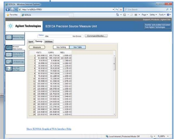
The web browser interface supports the B2900A's basic measurement capabilities (such as spot, sweep and pulsed measurement). Measurement results are displayed in a tabular format that can easily be copied into Excel for graphing and reporting.
