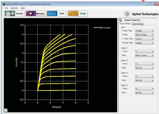
The built-in graph function supports both basic and advanced features (such as the family of curves shown here).
