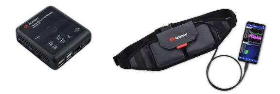
Nemo Diagnostic Module can be carried in a compact hip belt with a wired connection to the phone
