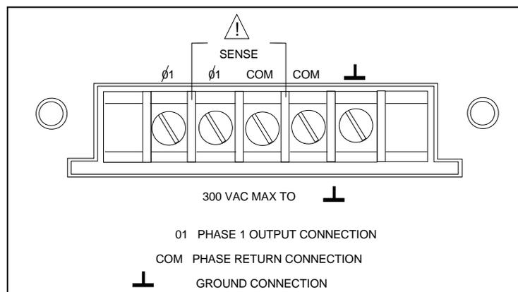
**Figure 2-4. Output Connections**
