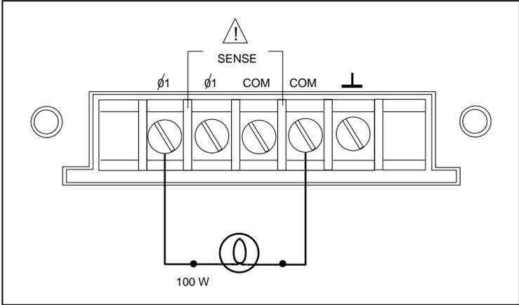
Figure 3-1.Verification Connections
