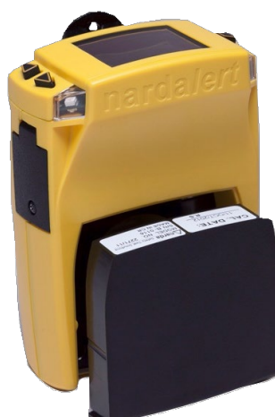
Fig. 4. Nardalert S3 mainframe shown with interchangeable sensor
