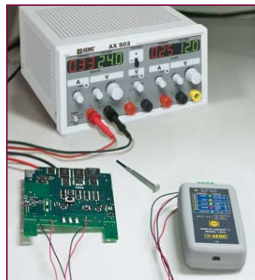
L432 recording two DC voltage supplies.
