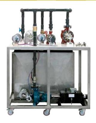
Mechanical section: the turbine under test is coupled to a permanent magnets DC generator simulating a variable brake. There is only one DC generator, which is moved and coupled to the turbine under test. The electrical power is dissipated in a resistive load. By measuring the generator electrical parameters (V, I, rpm) it is possible to calculate and plot the electrical power (Pe). The Efficiency % is then calculated with Ph and Pe.
