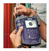
• Giving full control of the test set at both the local and remote ends lets users test and save results from either end of the test. This eliminates the need for additional technicians or for constantly walking back-andforth between local and remote test units.
